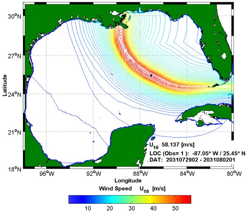
**Figure 14.4. Synthetic Hurricane No. 26 Wind Field Along Track**
