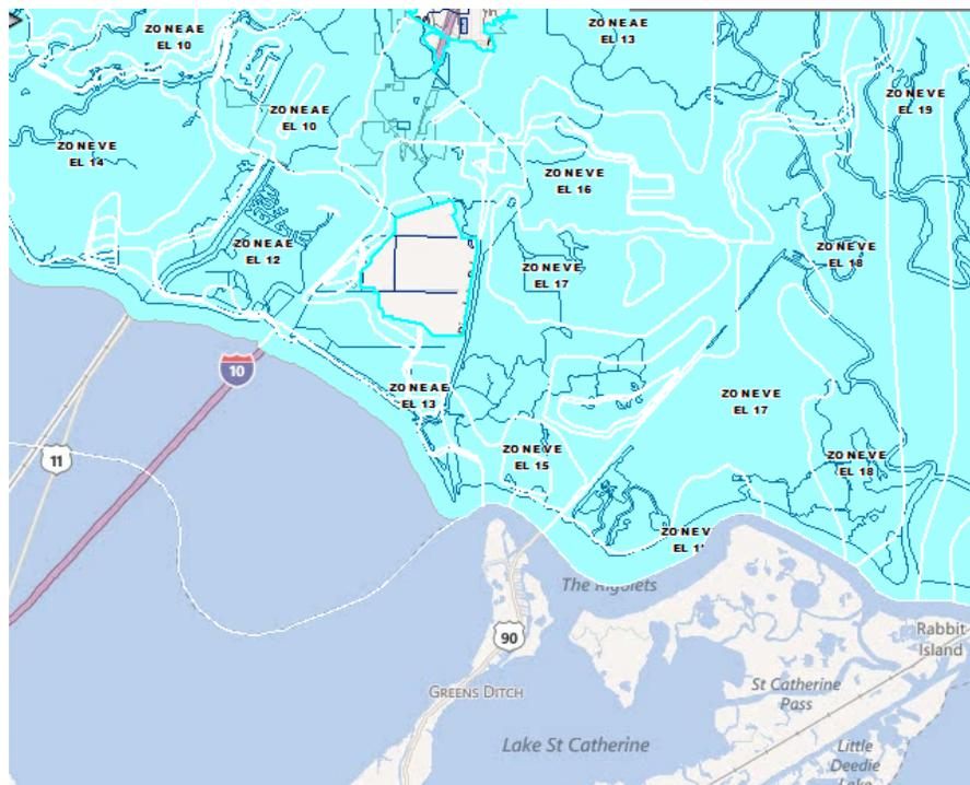
**Figure 14.10. Example of Wave Hazard Areas (VE Zones) Shown on FIRM**
