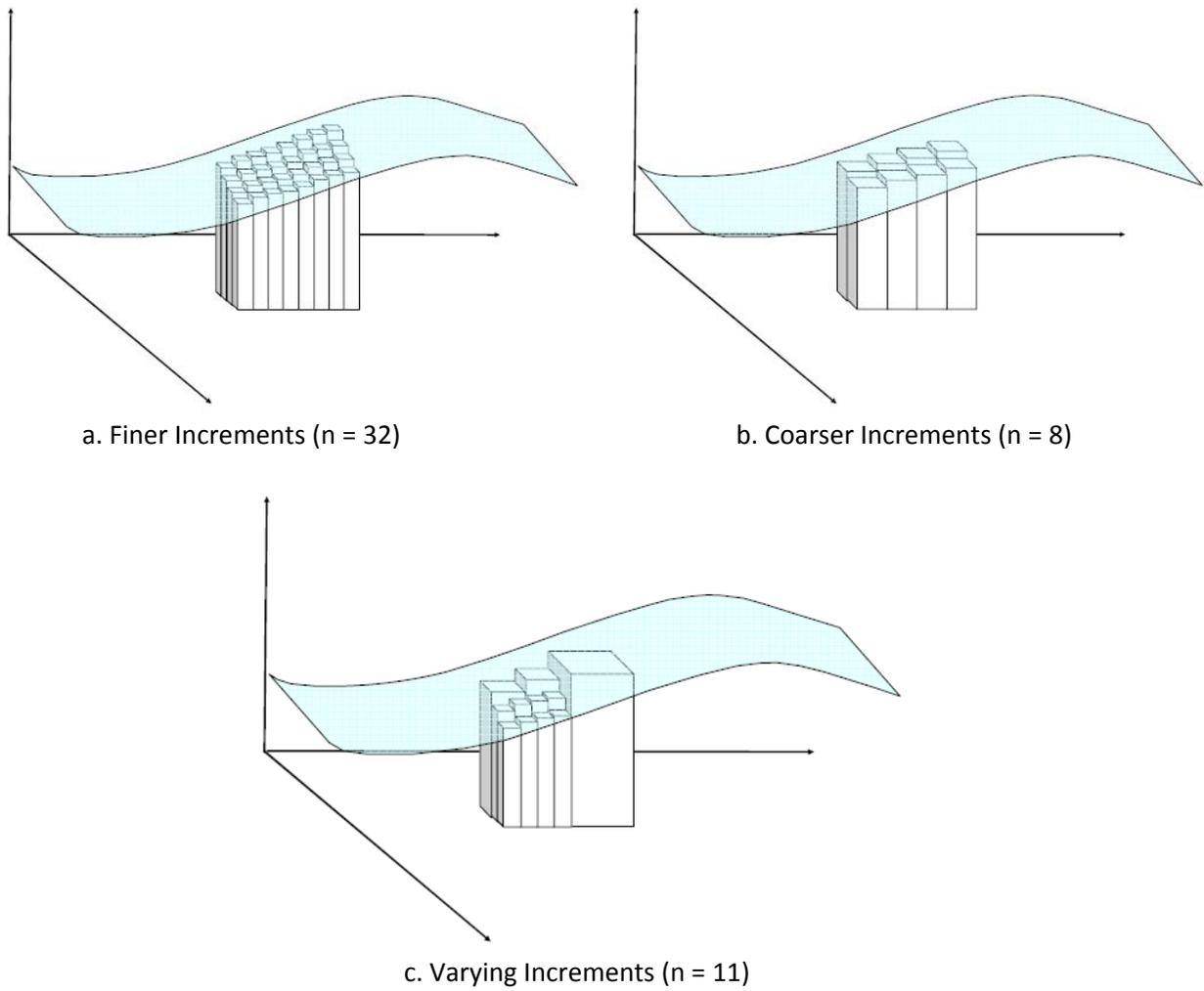
**Figure 13.1. Discretization of Volume Under a 3D Surface**
