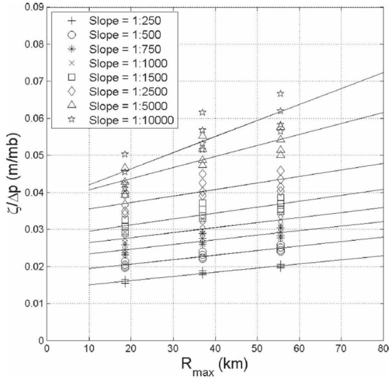
**Figure 13.4. Peak SWL versus  $R_{max}$  (normalized for CPD)**
