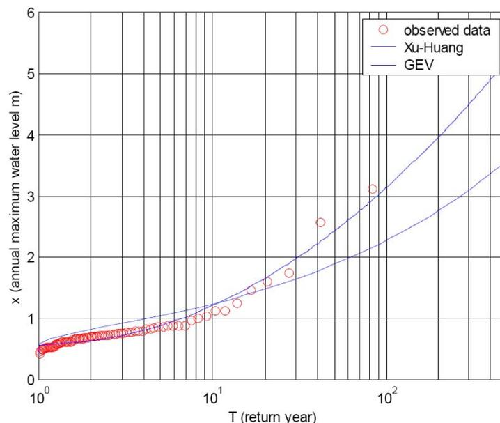
**Figure 12.1. Observed Annual Maximums at Pensacola Tide Station with GEV and Modified Distribution Functions**
