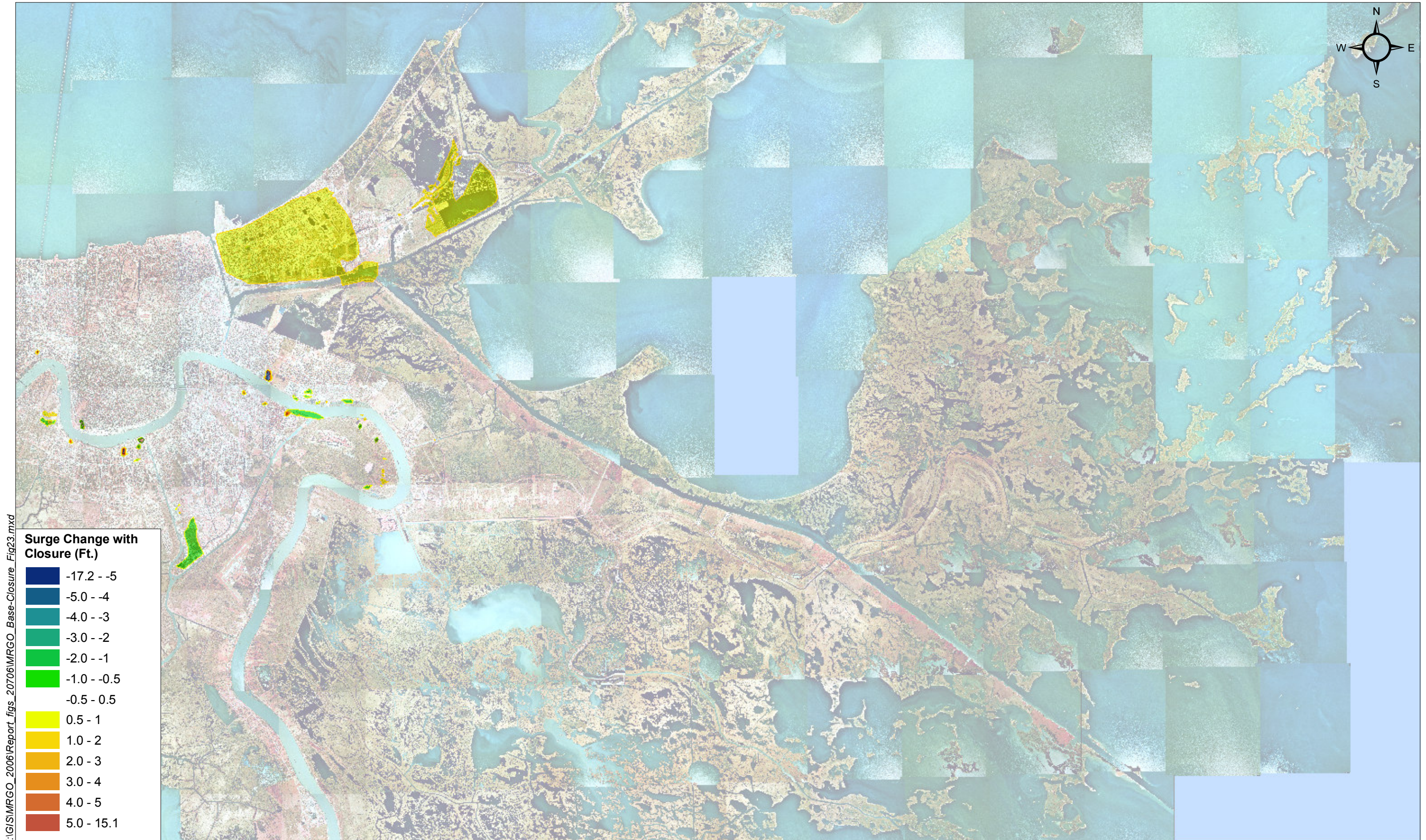
Figure 23 Difference in Maximum Water Surface Elevation for Hurricane Katrina, Baseline vs. Closed MRGO
